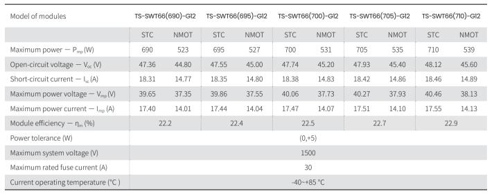
STC (Standard Testing Conditions): Irradiance 1000W/m<sup>2</sup>, Cell Temperature 25 °C , Spectra at AM1.5 NMOT (Nominal Module Operating Temperature): Irradiance 800W/m<sup>2</sup>, Ambient Temperature 20°C , Spectra at AM1.5, Wind at 1m/s
